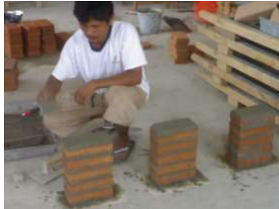
Figure 1 The Construction of Standard Test Form
